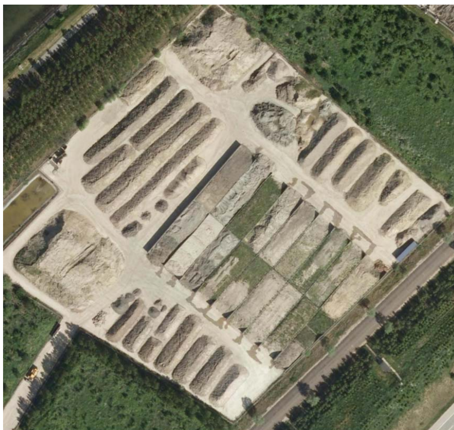
Figure 12: The same EK plant as pictured above after extension to a total of 18 bays and 2 years operation. In addition, the soil heaps outside the bays are treated by EK.
